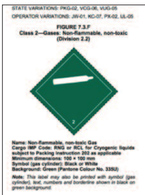
Fig. 2. Hazard label: Non-Flamm Gas e Criogenic Liquid
